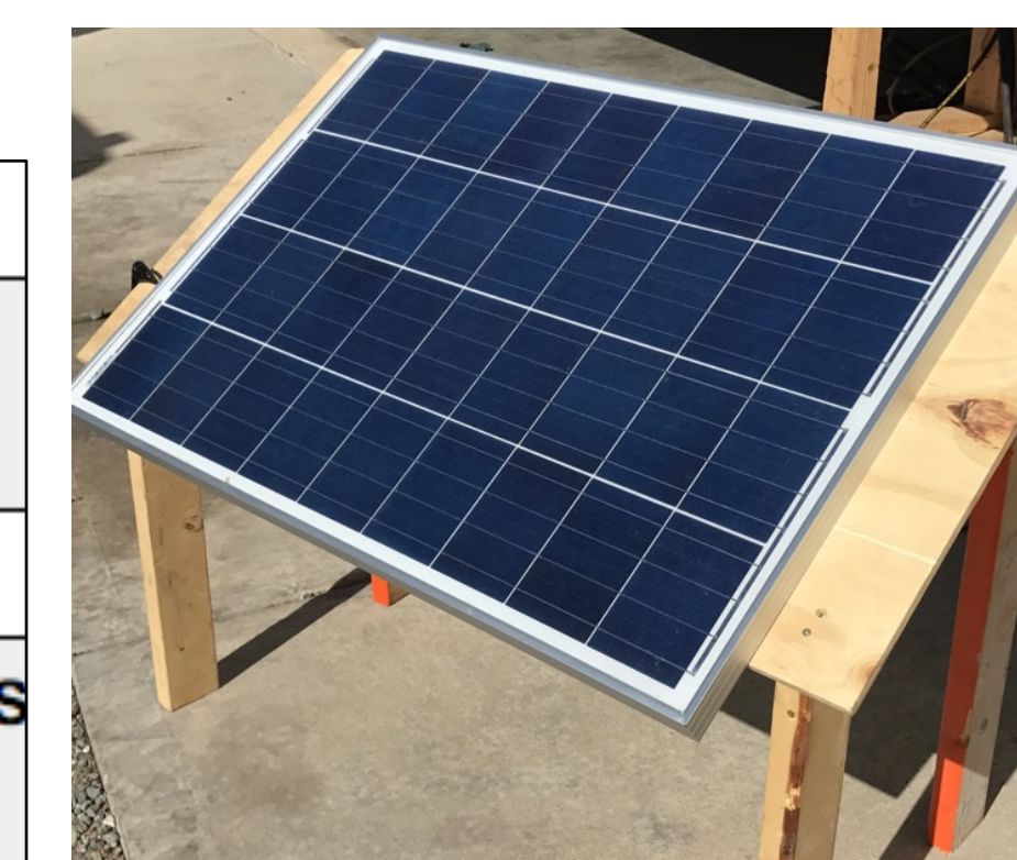
Solar panel mounted at an angle for optimum sun intensity
